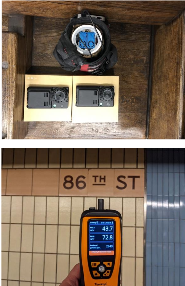
Figure 1: PurpleAir in canteen pouch for portability and two UPAS devices (top), actively collecting air quality data on a subway platform, and the Temtop (bottom) monitoring air quality at the 86th Street A/B/C/D platform.
